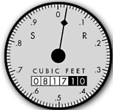
So, if by the time we read your meter the next time you had used 1,200 cubic feet of water, the new reading would be 82,910 (81,710 plus 1,200). The building use in gallons is calculated by subtracting the old number (81710) from the new number (82910) and multiplying by 7.48.
