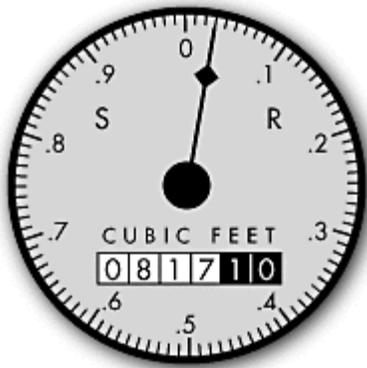
Stanford University's meters measure water in cubic feet (one cubic foot equals 7.48 gallons).
